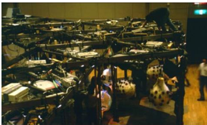
Figure 1: Overhead view of the Brain Opera Lobby truss structure, as being assembled before a Tokyo run in November 1996. All electronics are mounted at top the truss, leaving only the interactive interfaces (such as the Rhythm Tree bags at lower right) visible to the participants.
